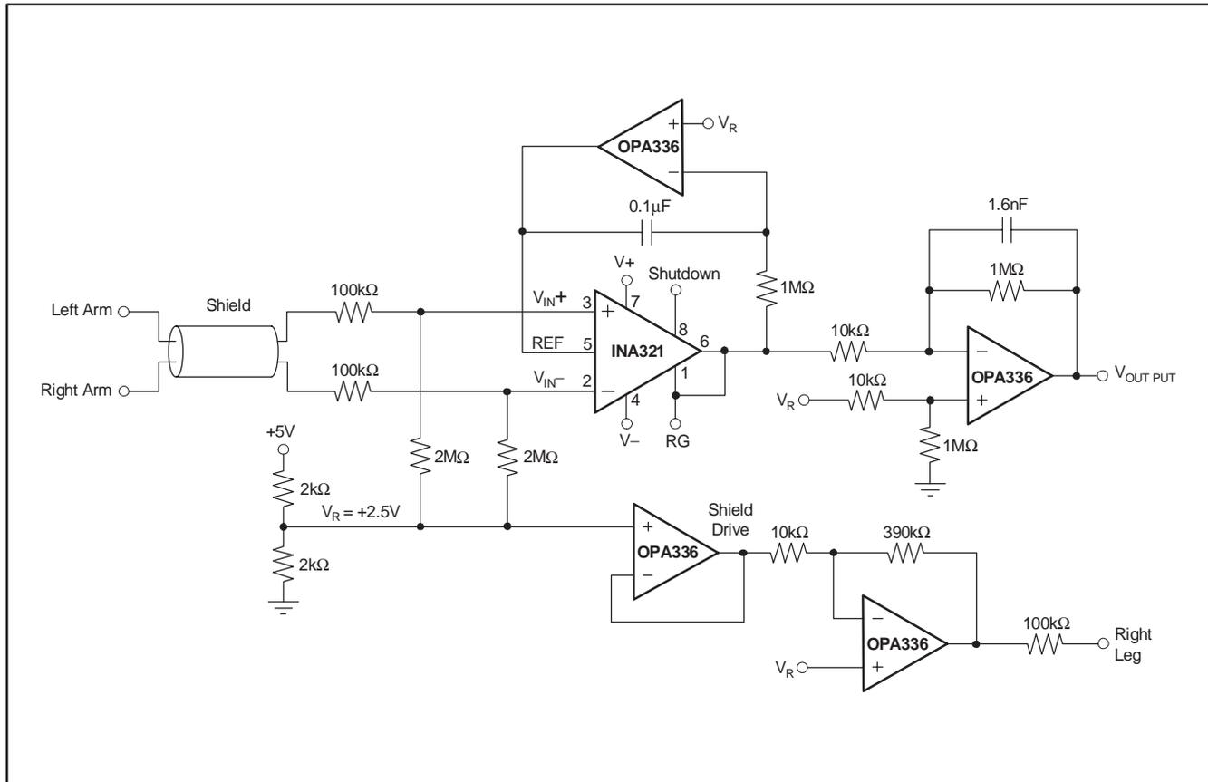
**Figure 9. Simplified ECG Circuit for Medical Applications**
