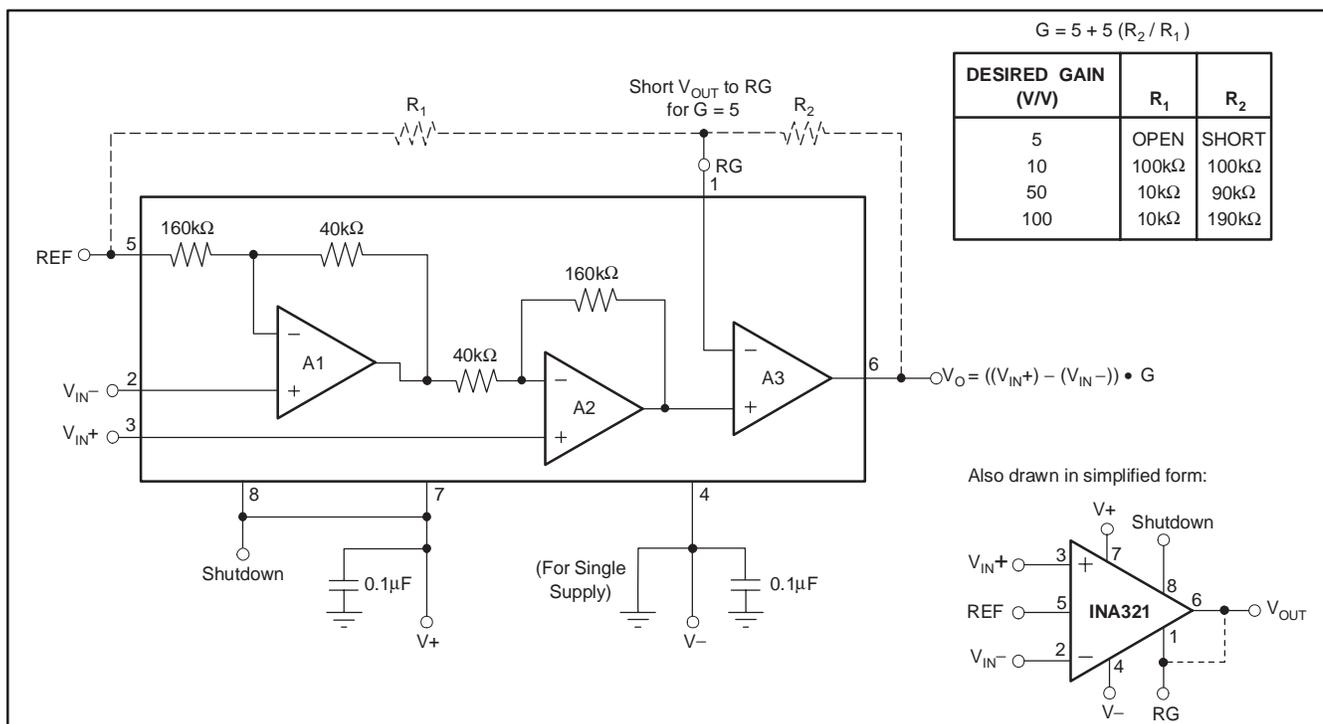
Figure 1. Basic Connections
