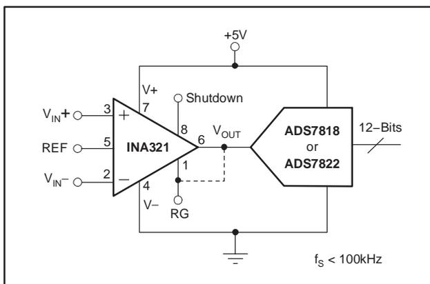
Figure 5. INA321 Directly Drives a Capacitive-Input, A/D Converter
