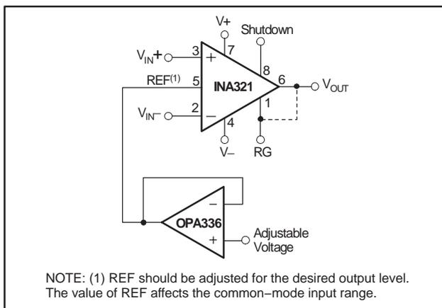
Figure 6. Optional Offset Trimming Voltage
